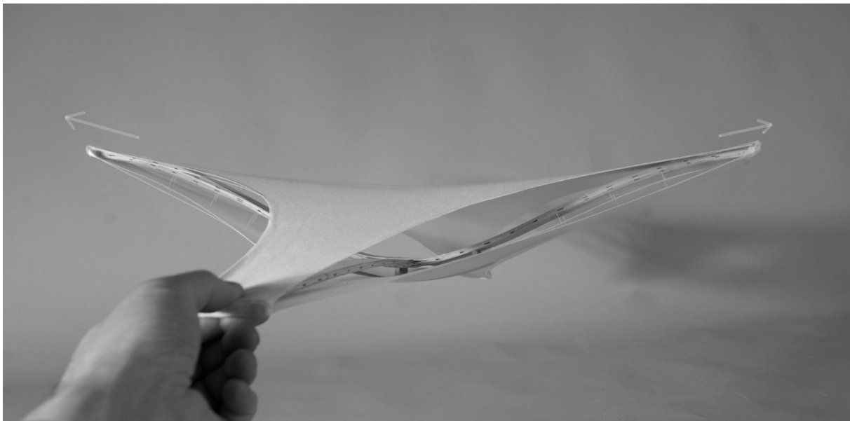
Figure 12: Case study 02 – the self-forming process while final-stressing the hybrid structure
